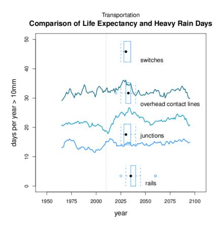
Figure 5: Box plots of the life expectancy of several components of the transport sector today, compared to the change of number of heavy rain days (11-year running mean) for three regions in Germany (Frankfurt, Munich, Berlin) for CCLM-C20/A1B model runs (Lautenschlager et al. 2009).
